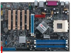
Attach the power LED, speaker, power and reset switch connectors to the corresponding pins. If you enable "Suspend Mode" item in BIOS Setup, the ACPI & Power LED will keep flashing while the system is in suspend mode.
