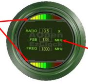
On the left circle area shows Ratio, FSB and frequency information about CPU. When the values are set to factory default, the light on the top and bottom of the circle will show green and it will vary as you change these CPU settings.
